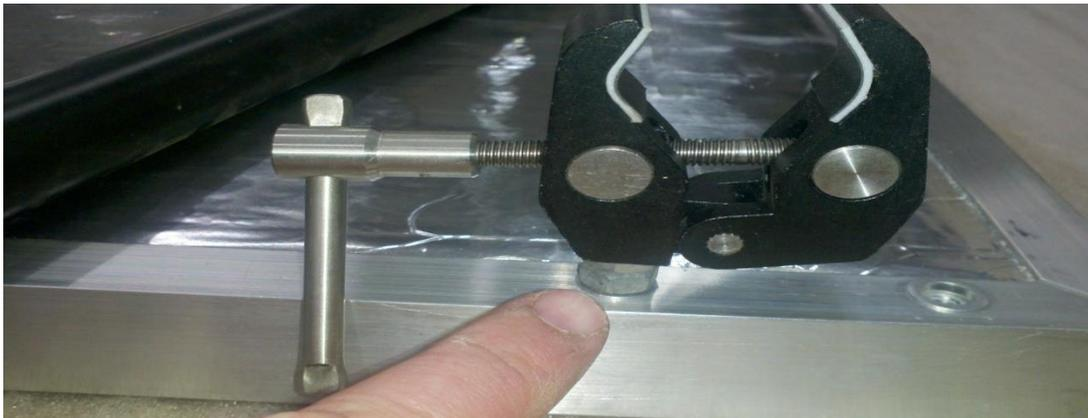
7) Lay cross bar into clamp jaws and gently tighten clamp. Do Not crush X-bar.
