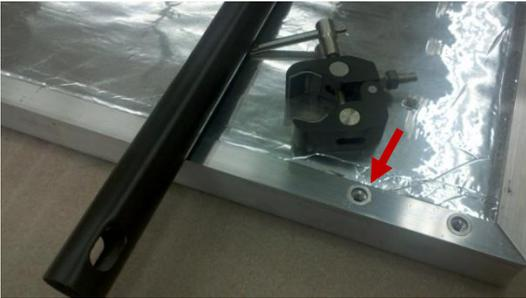
2) Line up 1/4-20 machine studs into holes by red tape.
